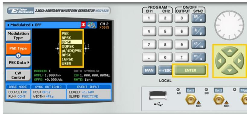
6. Following your selection, you will be able to configure the characteristics of the modulation with the modulation-type specific menu buttons that appear on the left-hand side of the panel.
