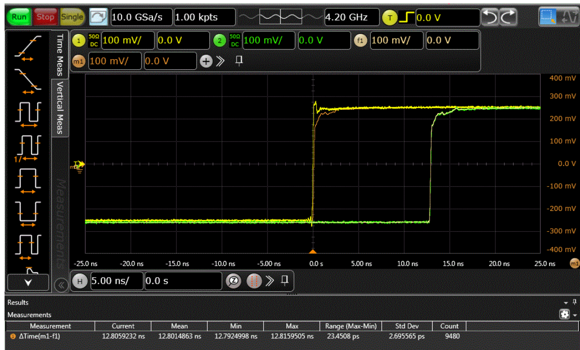
Figure 2-26 Marker Coarse Delay Expected Result and Scope Setup
