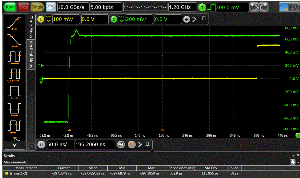
Figure 2-20 Trigger Jitter Test Expected Result and Scope Setup
