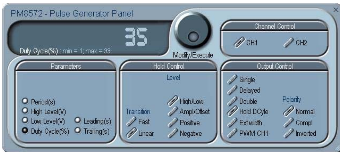
Figure 4-6, the Pulse Generator Panel with Linear Transitions and Hold DCycle Output
