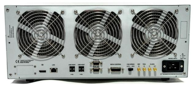
Figure 3.5 PXE21100 Rear Fan Exhaust
