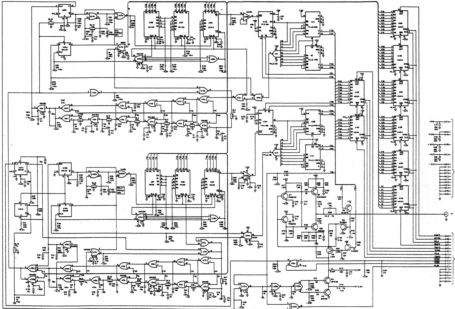
9-8 Pulse Width/Delay Board - Schematic Drawing
