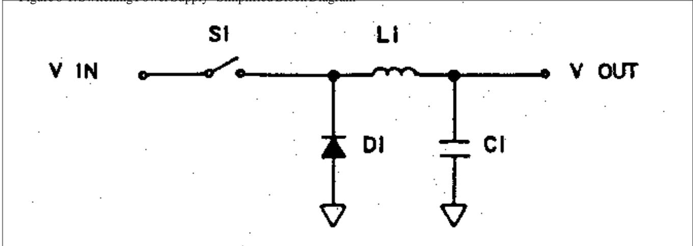
$$V_{out} = T_1 \times V_{in} / (T_1 + T_2)$$
