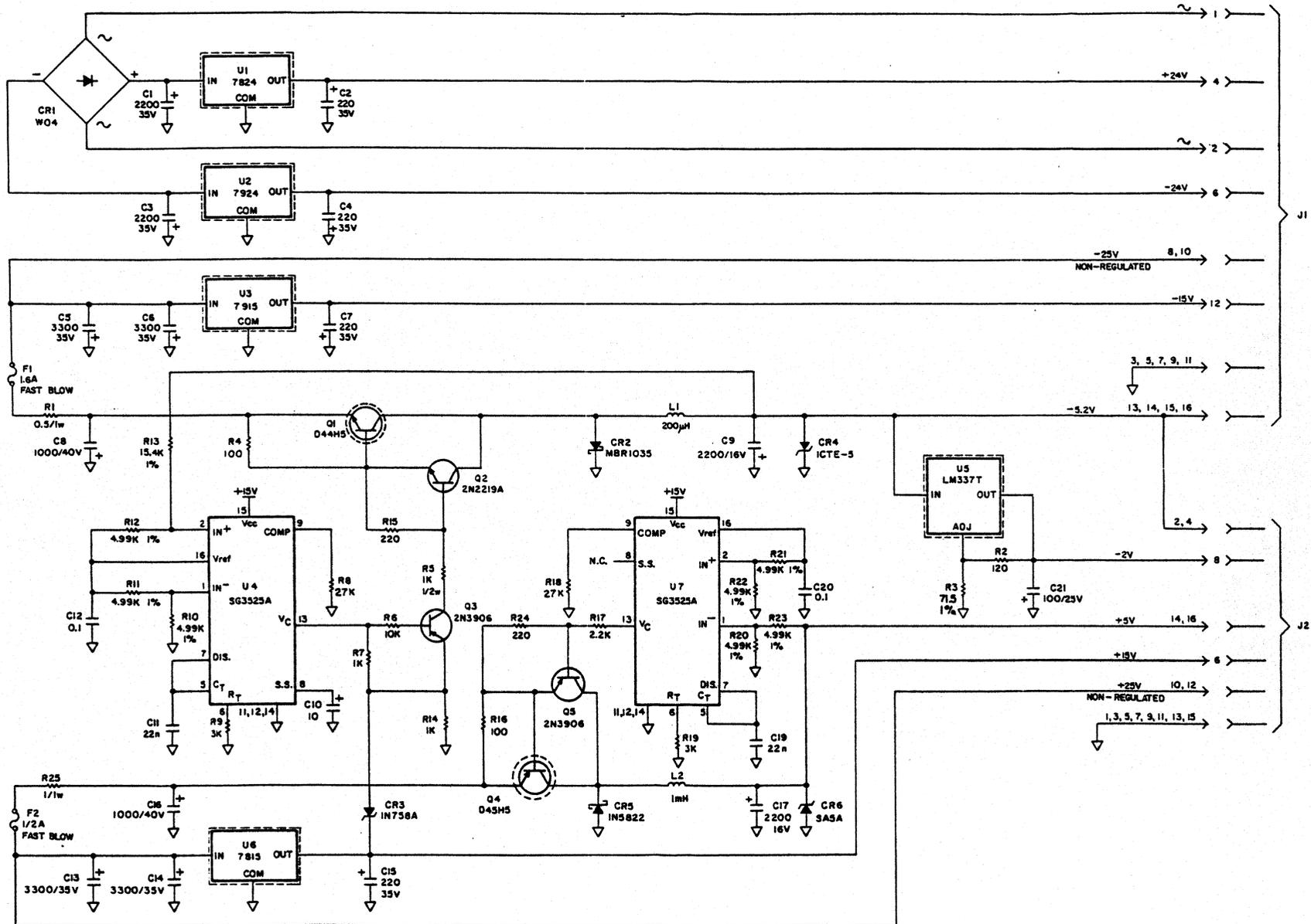
9-2 Power Supply Board - Schematic Drawing
