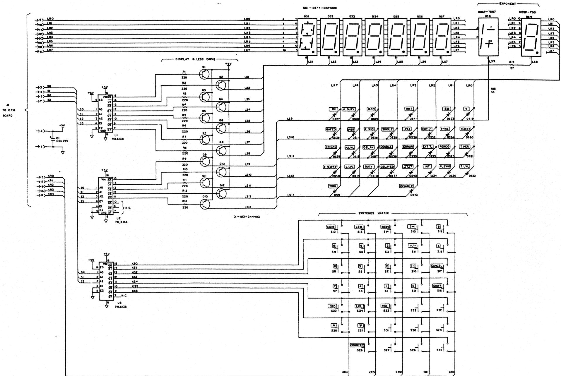
9-13 Display Board - Schematic Drawing
