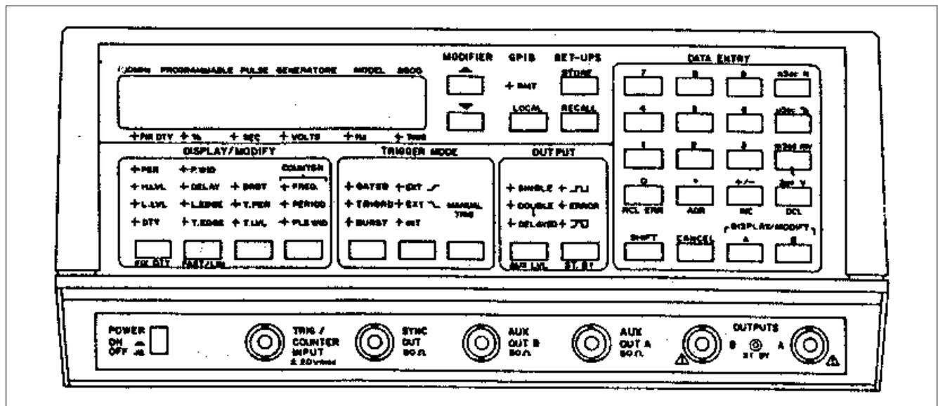
Figure 3-1. Front Panel Controls, Indicators and Connectors
