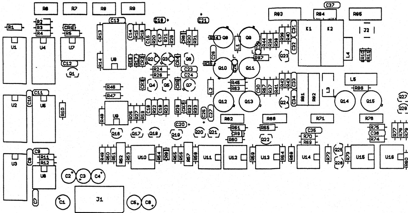
9-12 Output Amplifier Board - Assembly Drawing
