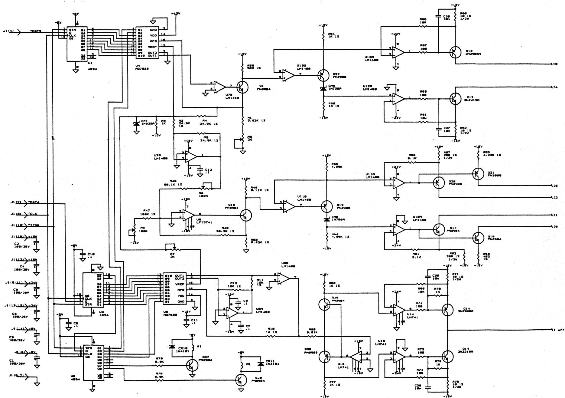
9-11 Output Amplifier Board Part 2 - Schematic Drawing
