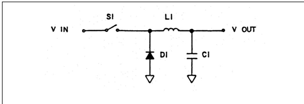
Figure 6-1. Switching Power Supply - Simplified Block Diagram
