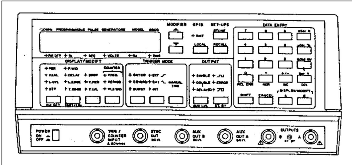
Figure 3-1. Front Panel Controls, Indicators and Connectors
