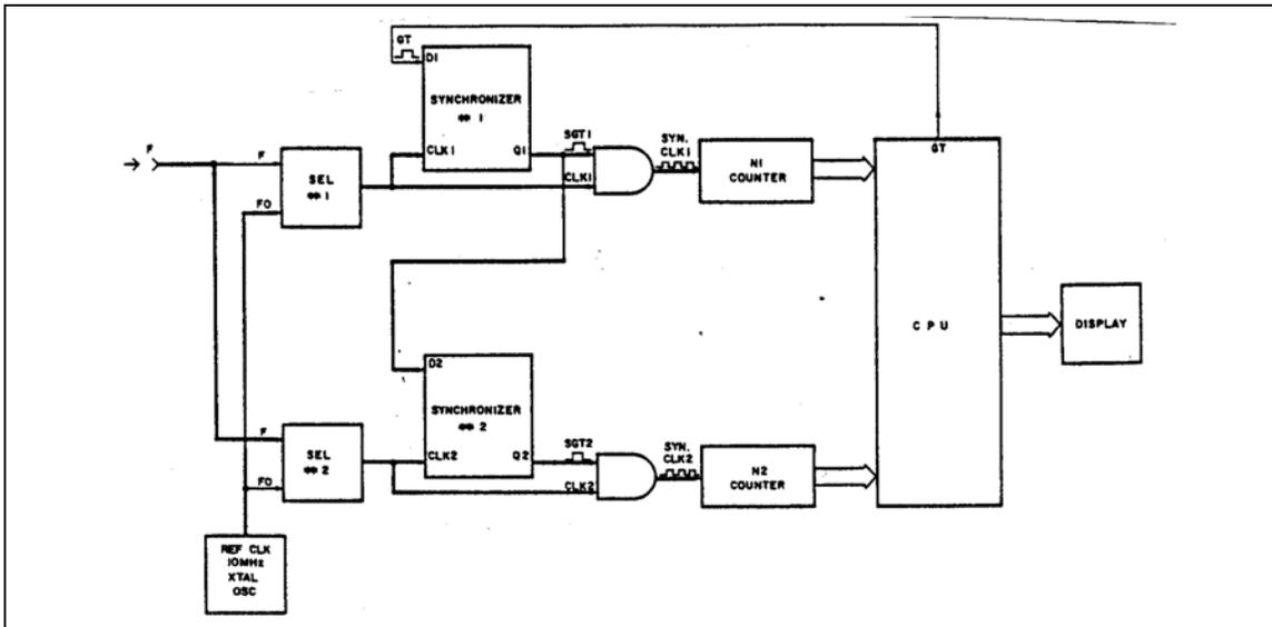
Figure 6-2. Conventional Frequency Measurement.
