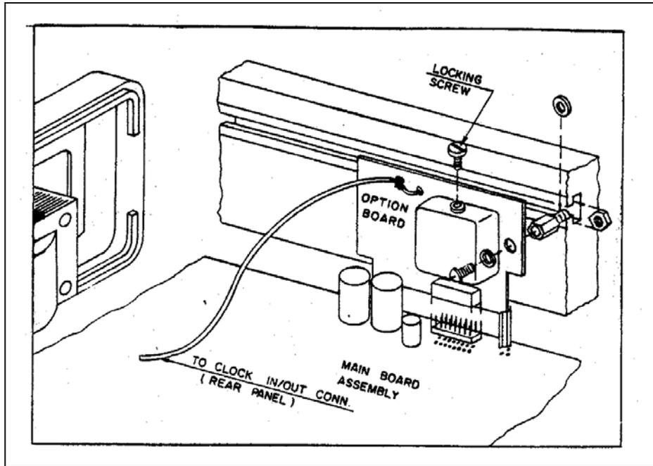
Figure 5-1. TCXO/Clock Multiplier Option Field Installation.
