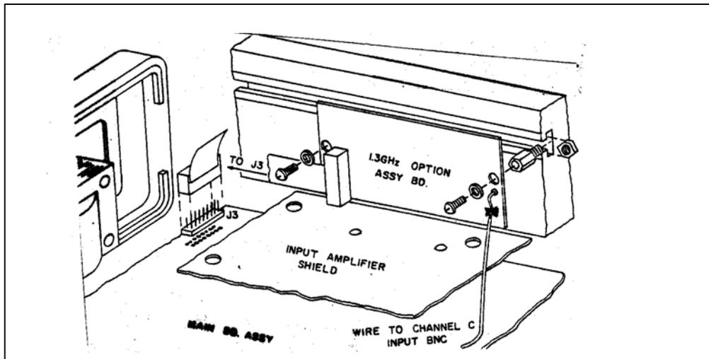
Figure 5-3. 1.3 GHz Input Option Installation
