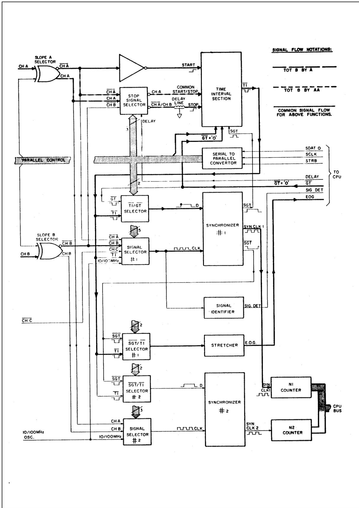
Figure 6-9. Totalize B By A and Totalize B By AA Signal Flow Diagram.
