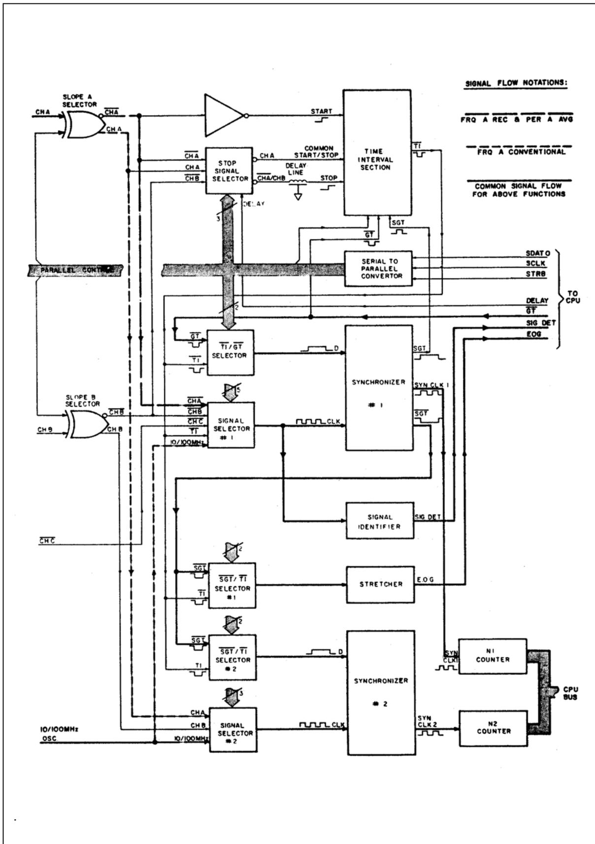
Figure 6-4. FREQ A Reciprocal/PER A Averaged and FREQ A Conventional Signal Flow Diagram.
