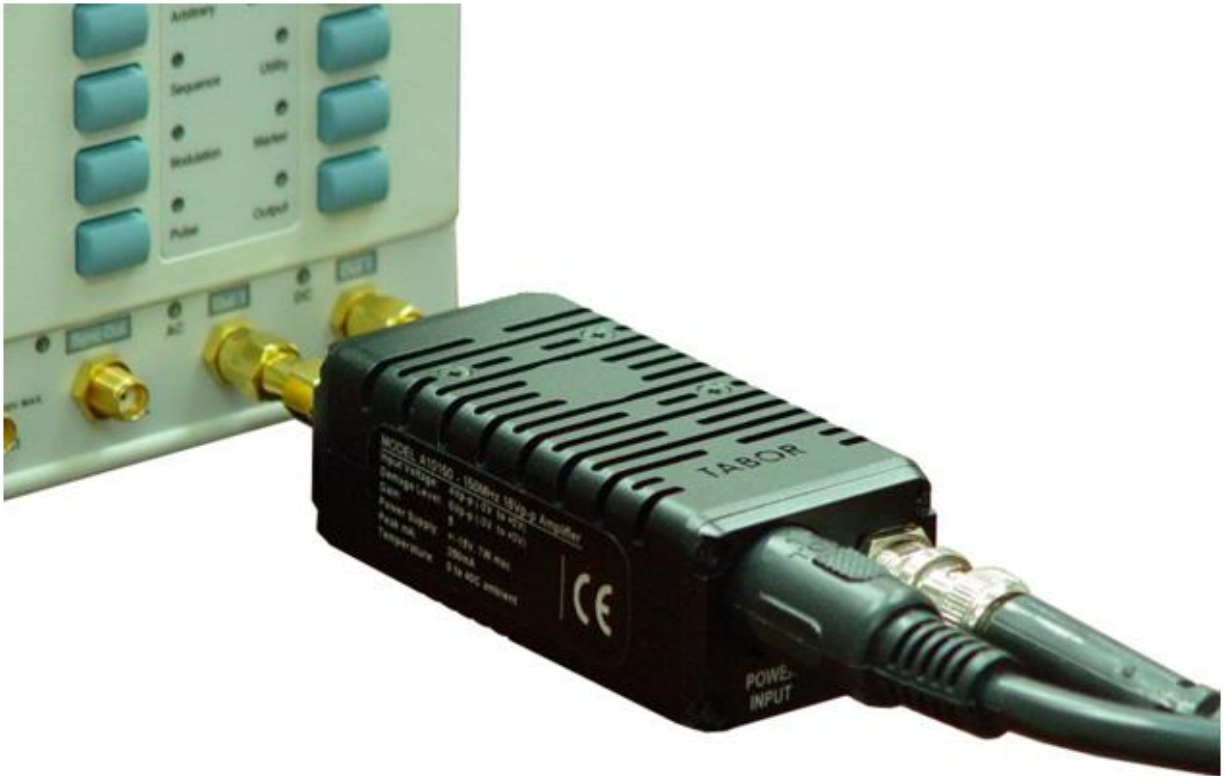
Figure 2.2 Connecting the A10150 to Tabor WX or WS8351/2 Unit
