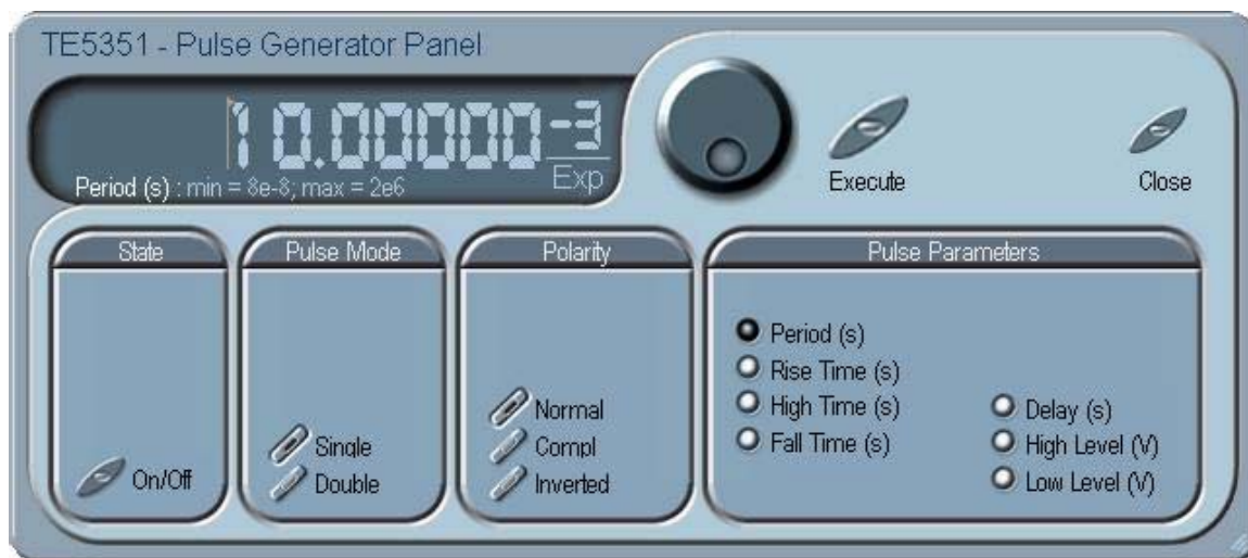
Figure 3-20, the Digital Pulse Generator Panel
