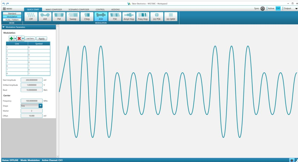
Figure 7.17 Quick Start Modulation ASK
