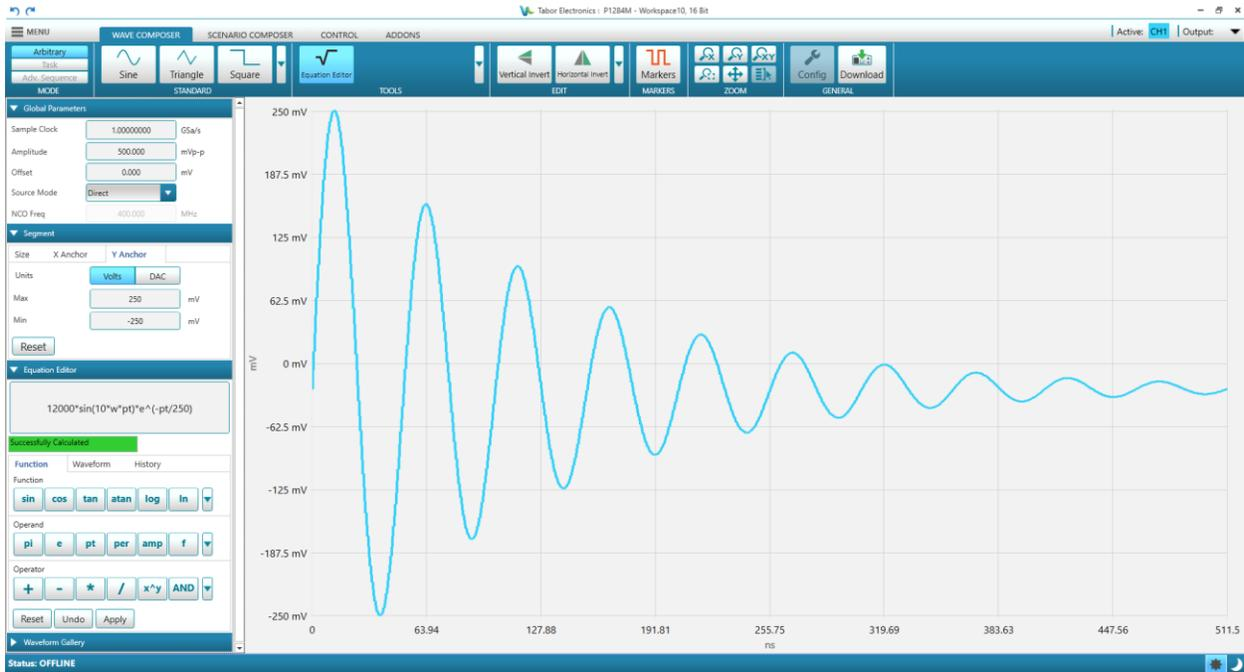
Figure 13.9 Equation Editor – Sine Wave with Exponentially Decay
