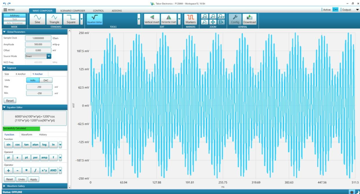
Figure 13.10 Equation Editor – 100 Cycles Sine Wave with Amplitude Modulation
