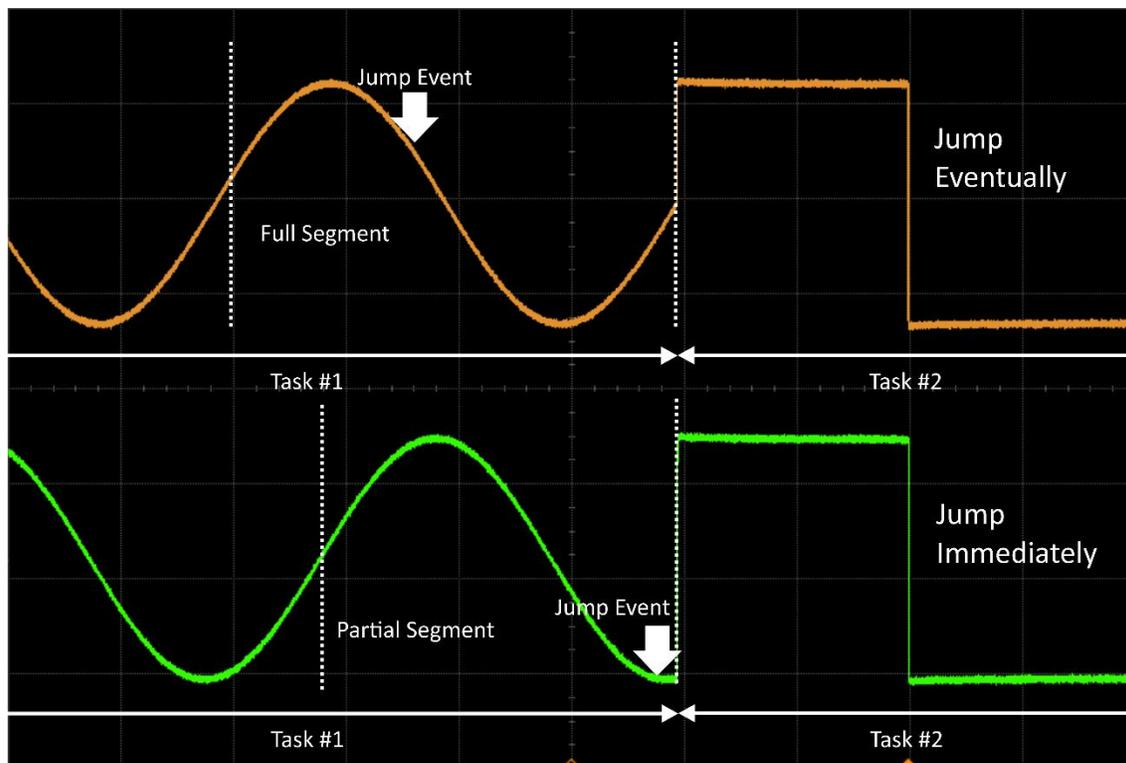
Figure 9.5 Different Types of Jumps. Jump Eventually (Top) and Jump Immediately (Bottom)
