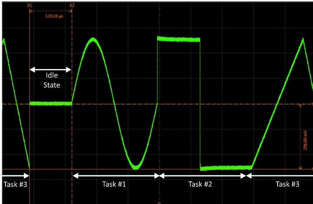
Figure 10.5 DC Level Idle State Associated to Task #1
