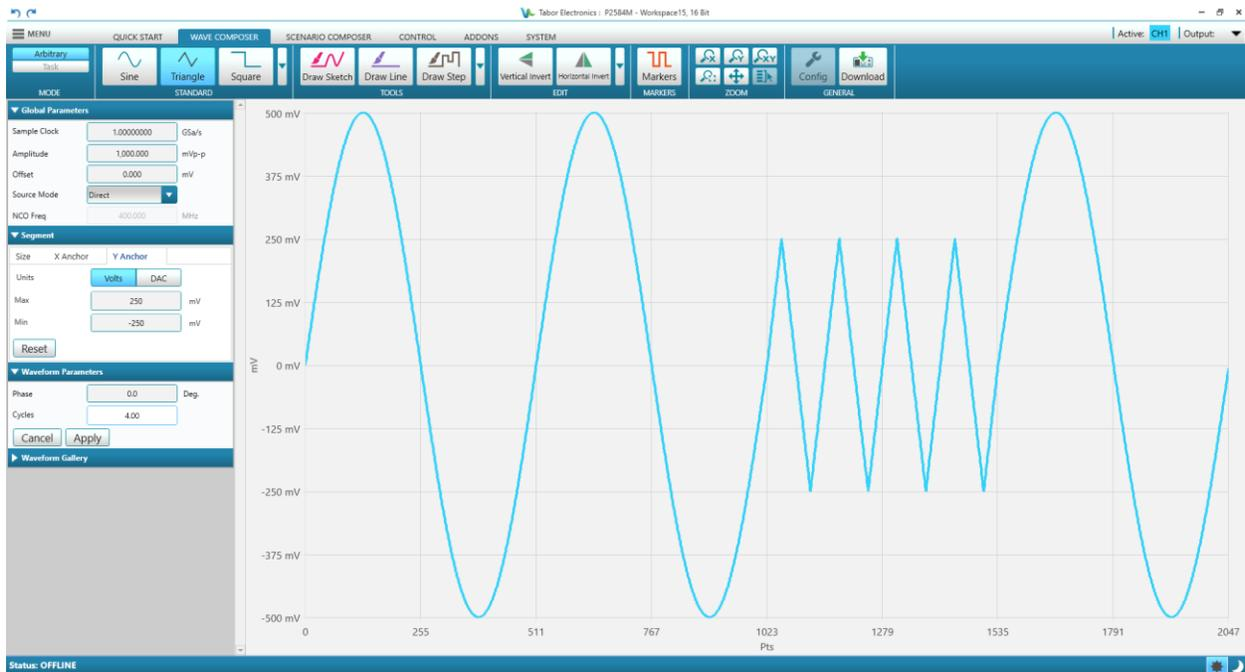
Figure 8.24 Sine Waves with a Triangle Waves (X Anchor Start 1,024, End 1535 Pts, Y Anchor Max 250, Min -250 mV)
