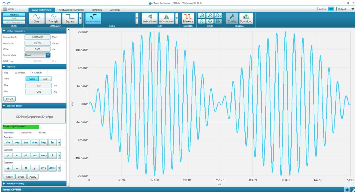
Figure 13.6 Equation Editor – Two Waves Modulation
