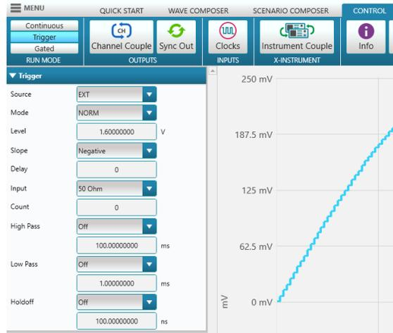
Figure 10.6 Trigger for SE- and WX-Series
