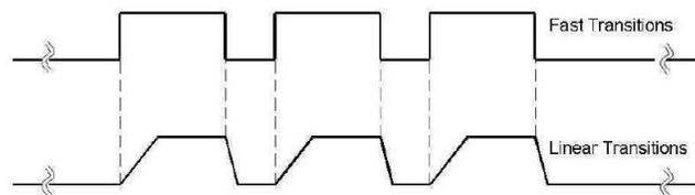
Figure 7.25 Quick Start Pulse Transition Types
