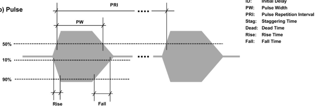
Figure 11.4 Explanation of Radar Pulse Parameters
