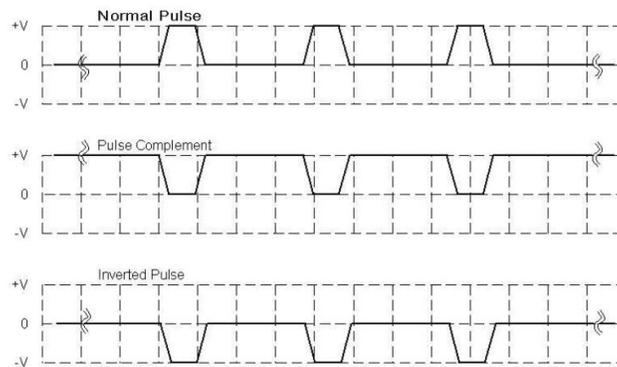
Figure 7.24 Quick Start Pulse Polarity
