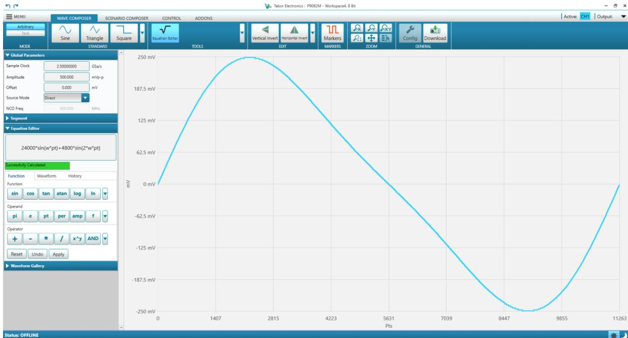
Figure 13.8 Equation Editor – Sine Wave with 20% Second Harmonic Distortion
