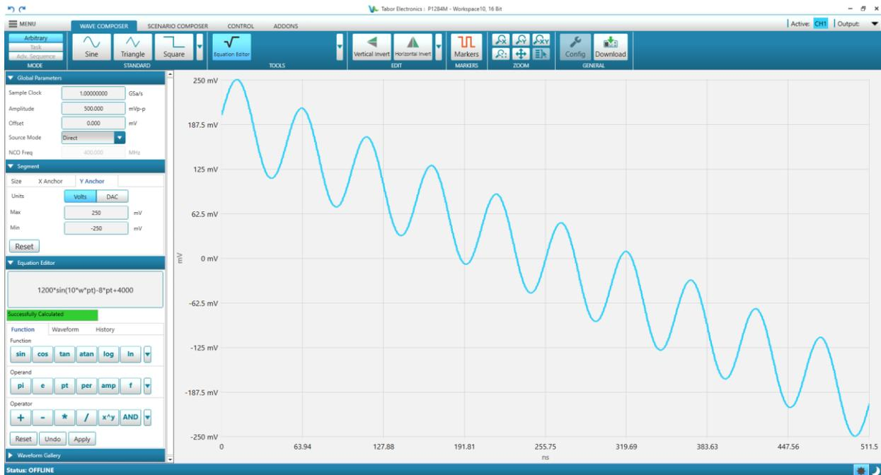
Figure 13.5 Equation Editor – Downslope 10 Sine Waves
