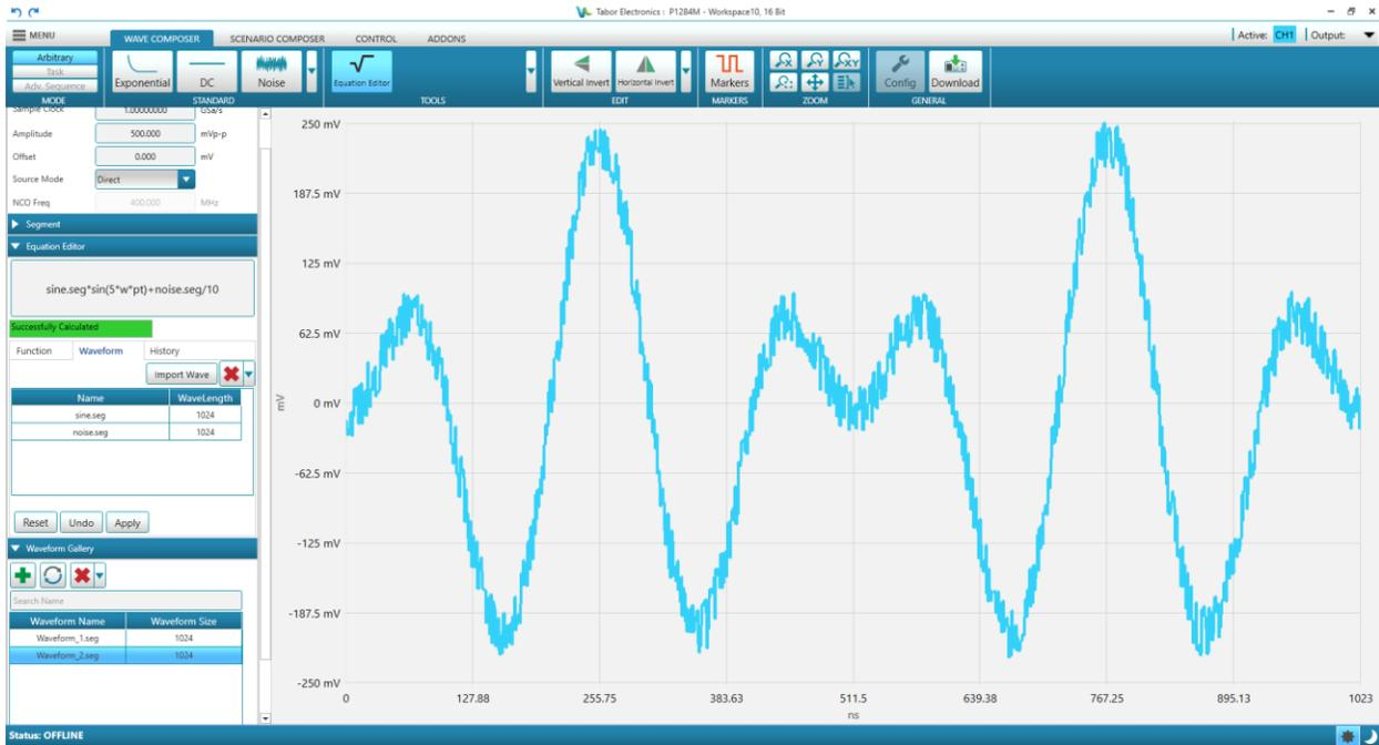
Figure 13.11 Equation Editor – Combining Waveforms
