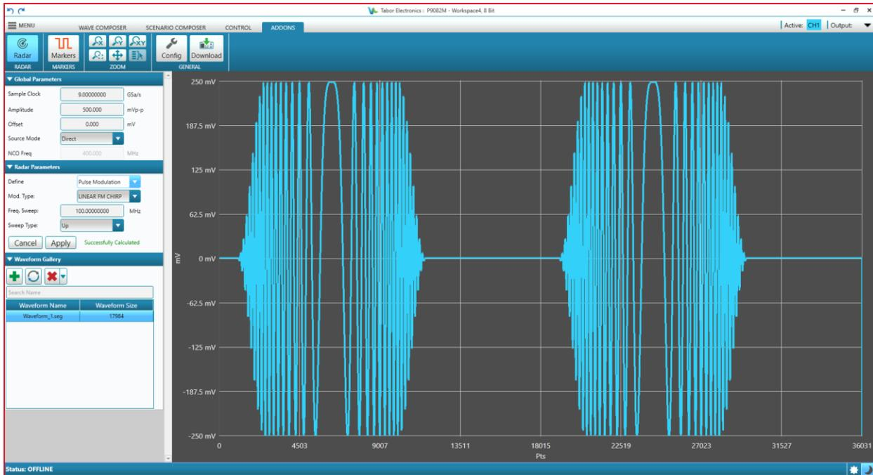
Figure 11.8 Baseband waveform (I component) for Linear FM Chirp Modulation
