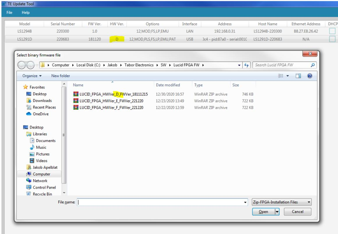
Figure 15.14 Select the FPGA Firmware File
