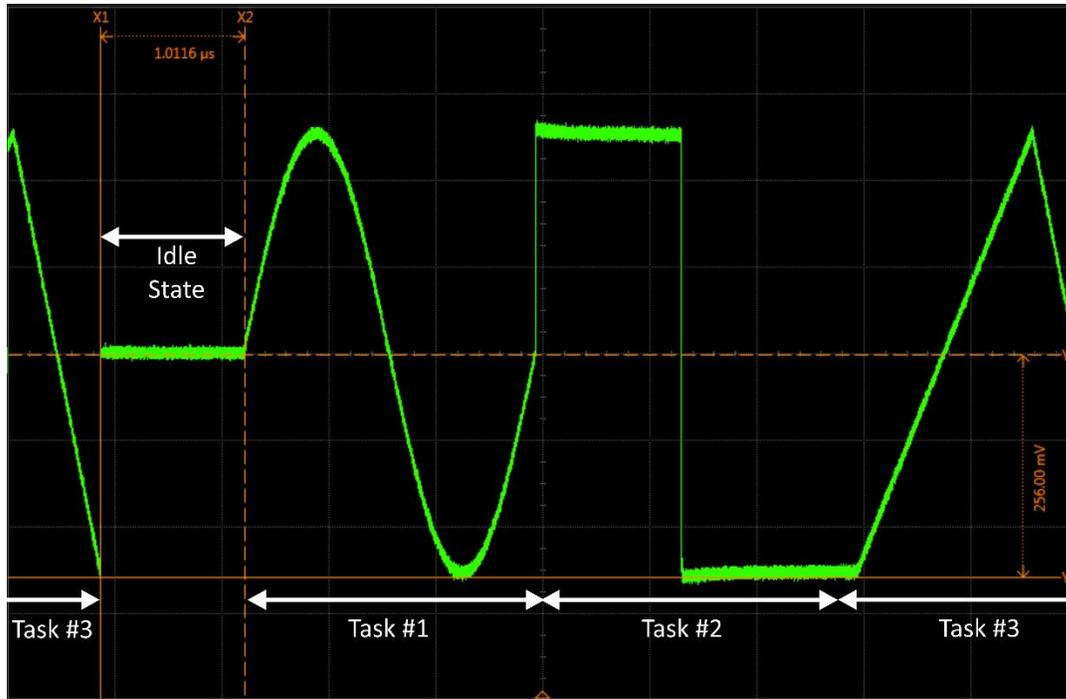
Figure 9.4 DC Level Idle State Associated to Task #1
