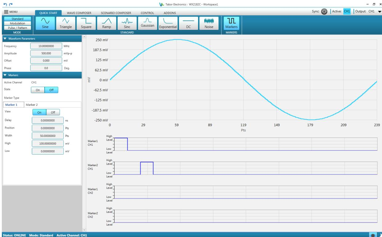
Figure 7.10 Sine Wave with Markers
