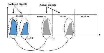
Figure 10.18 DDC RF Signals Over Multiple NZ
