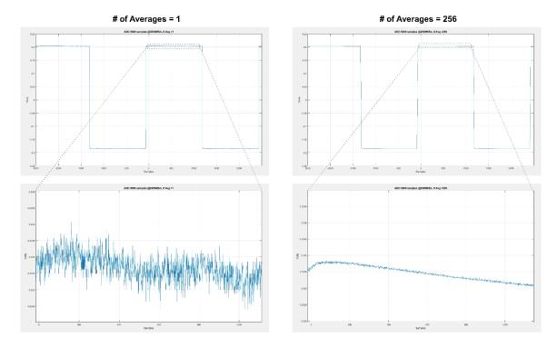
Figure 10.13 Averaged Acquisitions of Repetitive Waveforms (Right) Results in Lower Noise and Higher Resolution Acquired Waveform Respect to Non-Averaged Waveforms (Left)
