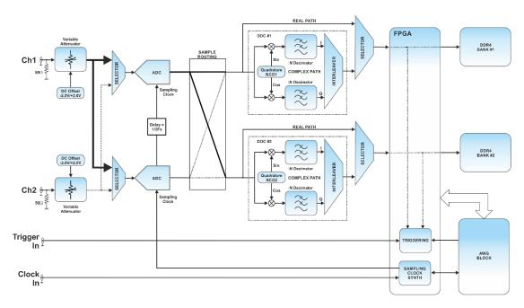
Figure 10.3 Digitizer Section Block Diagram for SINGLE Mode
