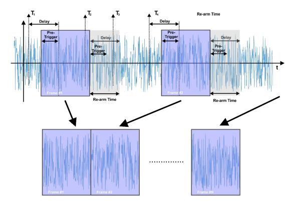
Figure 10.7 Structure of a Multi-Frame Acquisition
