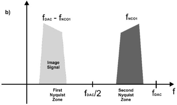
Figure 8.5 I/Q Effects of Setting the NCO Frequency within the First (a) and the Second (b)
