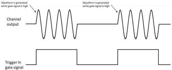
Figure 9.1 Output Signal with Gate Type Trigger
