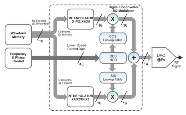
Figure 8.1 IQ Modulator Block Diagram
