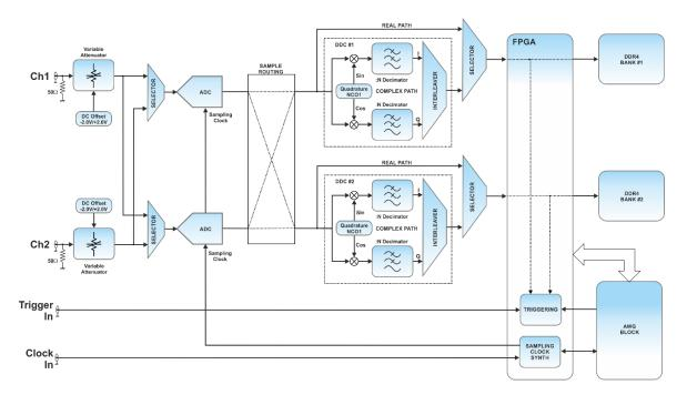
Figure 10.1 Digitizer Section Block Diagram for DUAL Mode
