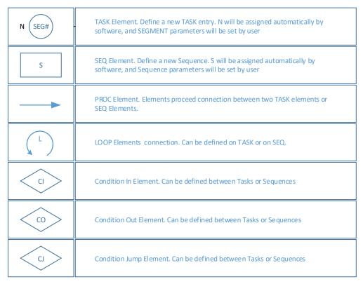
Figure 6.1 Type of Blocks Implemented by the Task Table
