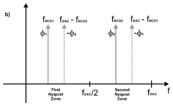
Figure 8.3 Effects of Setting the NCO Frequency within the First (a) and the Second (b) Nyquist Band
