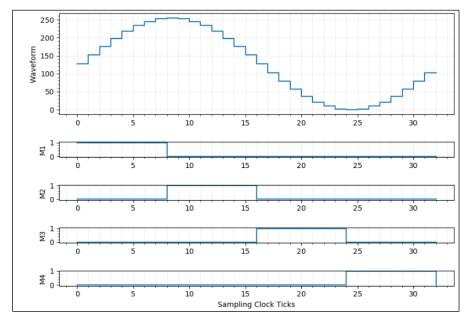
Figure 7.1 9 GS/s Model - 32 Waveform Points and 4 Marker Points
