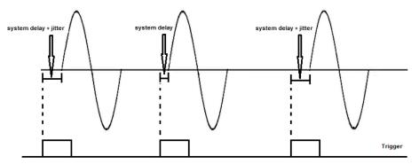
Figure 9.4 Trigger Jitter and System Delay
