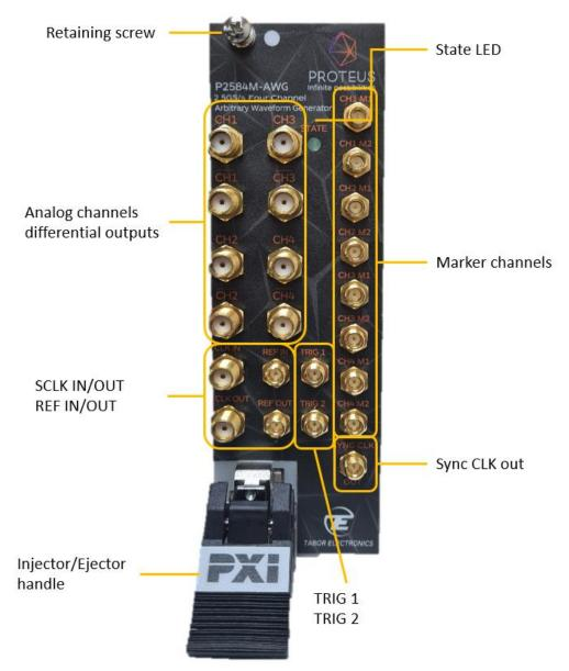
Figure 2.4 P2584M Front Panel
