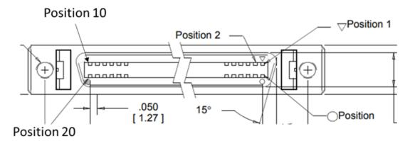
Figure 13.1 MDR Connector Pin Numbering
