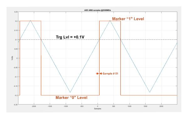
Figure 10.12 Trigger Signal Applied to Ext Trigger Input and Ch1. The Red Trace Shows the Contents of the LSB of the Acquired Waveform in the Marker Mode and the Actual Position of the Trigger Event
