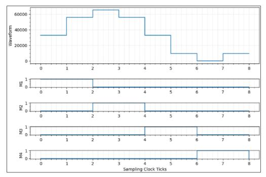
Figure 7.3 P2582M Model 8 Waveform Points and 4 Marker Points
