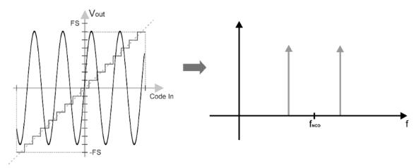
Figure 8.10 DAC Range Adaption to Avoid the Residual Carrier Impairment in the Output as Seen in (a)
