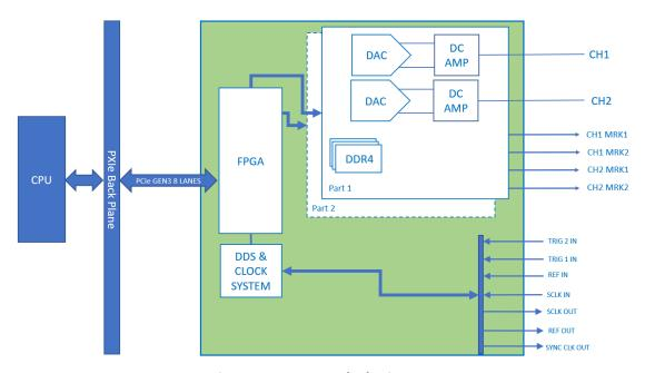
Figure 4.2 Proteus Block Diagram
