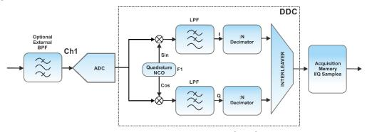
Figure 10.16 Digital Down-Converter (DDC)
