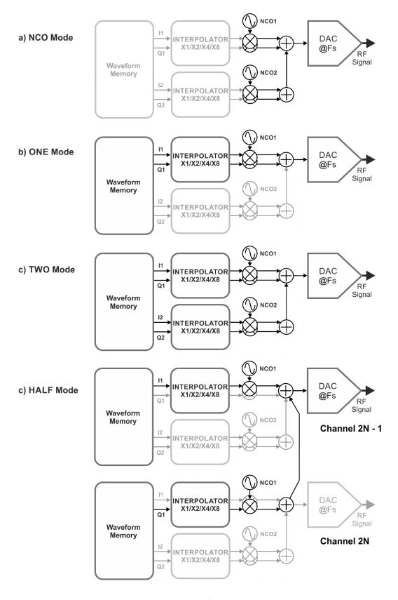
Figure 8.2 DUC Working Modes for Proteus P948X and P258X
