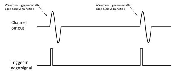
Figure 9.2 Output Signal with Positive Edge Type Trigger
