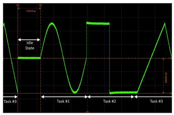
Figure 6.3 DC Level Idle State Associated to Task #1
