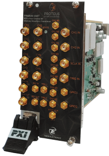
4 Direct to RF Synchronous Outputs, 2 RF Digitizers
