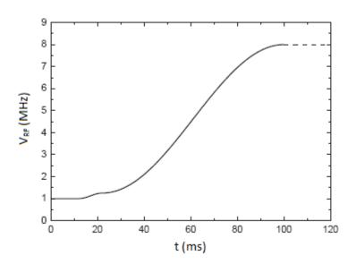
Figure 1: RF "Ramp" Used to Trap Supercooled Atoms
