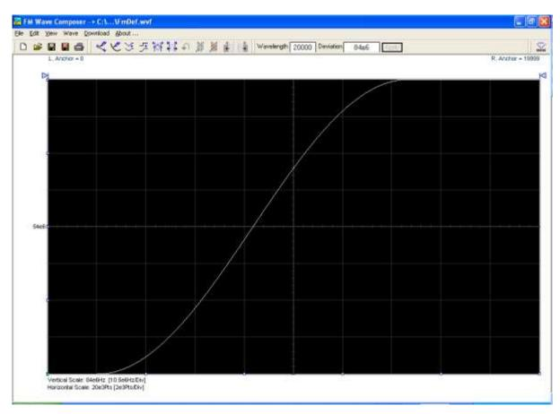
Figure 2: Tabor Wave Composer Tool for Arbitrary Wave Design
