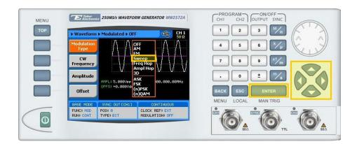
**6.** Following your selection, you will be able to configure the characteristics of the modulation with the modulation-type specific menu buttons that appear on the left-hand side of the panel.
