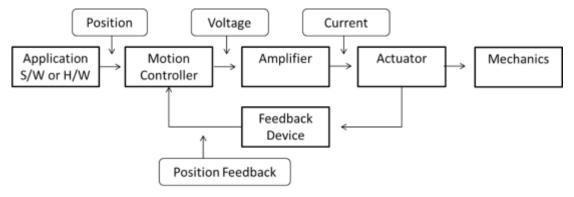
Figure 1: Motion Control Block Diagram
