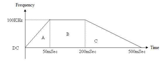
**Figure 2: Control Signal Diagram**
