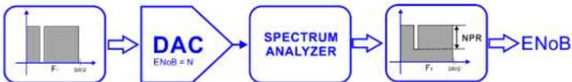
Figure 3.1: There are several methods to obtain the  $ENoB$  (Effective Number of Bits) parameter. Some of them (a, b, c) try to measure SINAD directly using multiple methodologies. Others, like the NPR (Noise Power Ratio) method (d) show the  $ENoB$  parameter indirectly. Test signals are also different. The SINAD based methodologies use single frequency sinewaves while the NPR method uses wideband random-like test signals.
