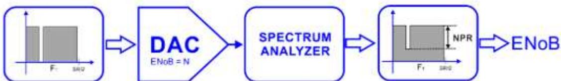
Figure 2.1: There are several methods to obtain the  $ENoB$  (Effective Number of Bits) parameter. Some of them (a, b, c) try to measure SINAD directly using multiple methodologies. Others, like the NPR (Noise Power Ratio) method (d) show the  $ENoB$  parameter indirectly. Test signals are also different. The SINAD based methodologies use single frequency sinewaves while the NPR method uses wideband random-like test signals.
